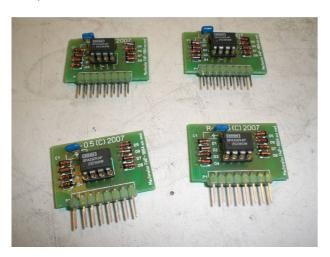
Here you see the pcb with the, in this case, OPA2604 and the 8 protection diodes. Please note that re rev numbers can differ since we always try to improve our products so every time a change to the design / pcb is made we go up a level.
